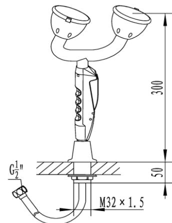
**Instructions:** When in use, withdraw the main body of the eye washer from the table holder, push the push button with your thumb and push forward at the same time, the switch valve opens and locks the water flow, allowing you to rinse. After the rinse is completed, pull back the push button and release, the switch valve closes, and then reset the main body of the eye washer to the table mount.
