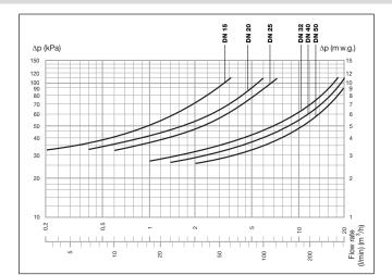
This chart shows curves at a 800kPa inlet pressure and 300kPa set pressure; curves for other settings are similar. The curve shifts slightly to the left for a
