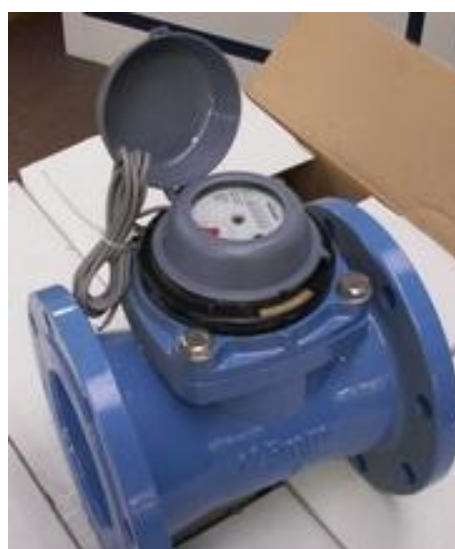
4) Close the cup letting the wire out through the slot and close it with the seal
