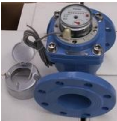
4) Insert the sensor in the position shown (in no case insert the sensor in any other position)
