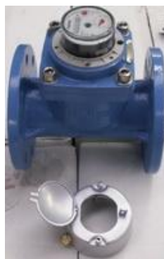
2) Remove the metal ring using a 4 mm allen wrench
