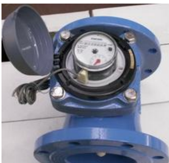
3) Insert the sensor in the position shown in the pic. (in no case insert the sensor in any other position)
